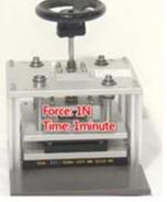
1) Press OCTA Window using Window pressing JIG.
