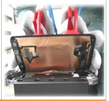
1)Detach the Bracket carefully from the LCD using Glass absorber and holder.
