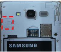
1) Assemble LCD unit on the Rear case.
