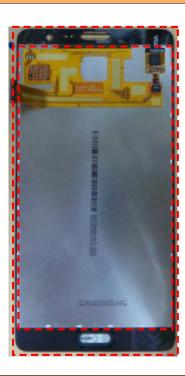
1) Attach LCD tape on the LCD unit using LCD tape attaching JIG.
