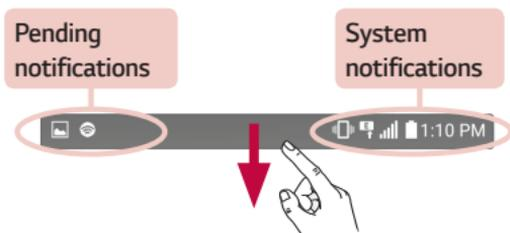
The icons displayed at the top of the screen provide information about the status of the device. The icons listed in the table below are some of the most common ones.
