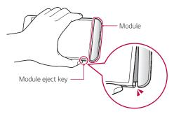
2 Grab the middle of the ejected module and pull it out from the device.
